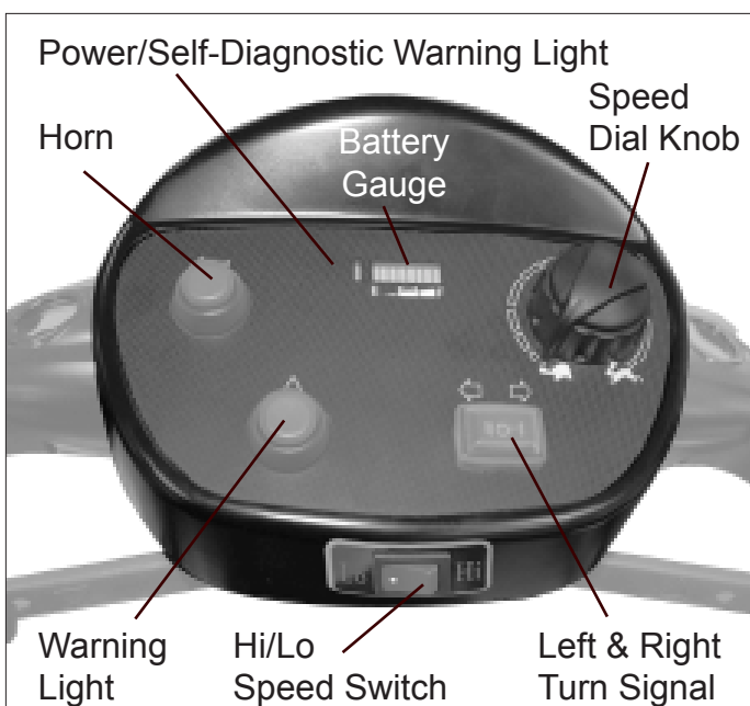
Figure 2 - Top Control Panel
